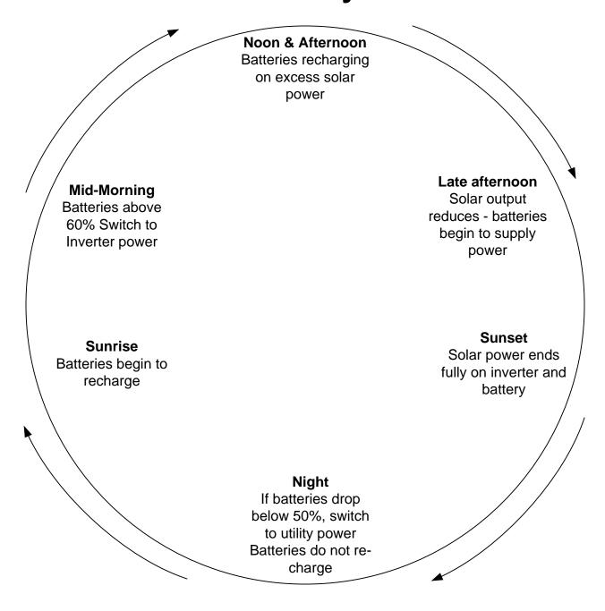
Overnight – Mi-Grid monitors the utility. If the utility feed stops supplying power, the system will immediately switch to inverter battery power. The generator will then turn on automatically and begin recharging the batteries. At 75% charge, the generator will shut off and not come back on unless the batteries go below 50%. If the utility is restored, Mi-Grid will switch back to utility power, generator will shut off.
